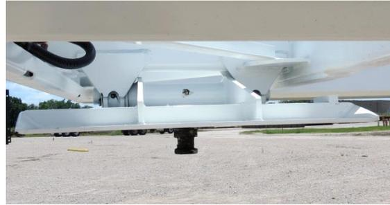
PCI manufactures heavy-duty 5<sup>th</sup> wheel plates/kingpins from  $\frac{3}{8}$ " plate to offer greater security; a single pin in the kingpin's solid housing offers greater durability and longevity for your investment.
