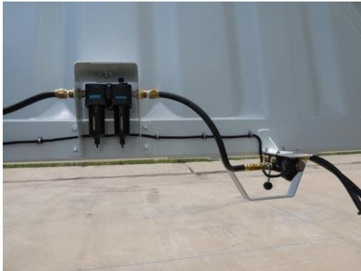
All wiring is loomed and secured to the trailer to prevent damage from exposure and falling debris.
