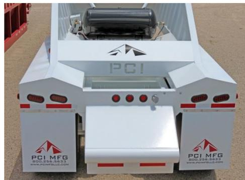
Sloped fenders prevent debris and water accumulation.
