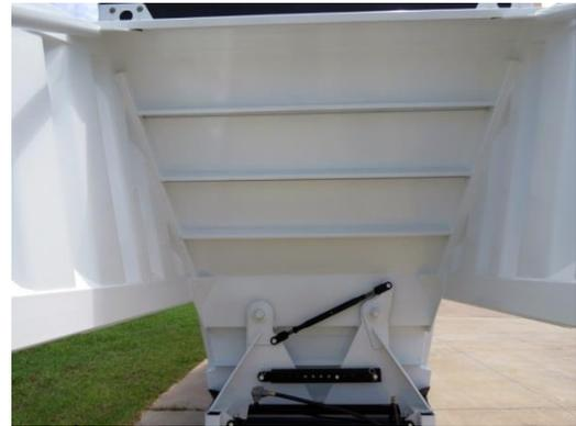
Where the corrugations meet the vertical members, many manufacturers leave holes to reduce the weight of the trailer. PCI kept the trailer weight low while still sealing these holes to help prevent rust-out.
