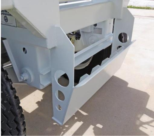
Fabricated from  $\frac{3}{8}$ " plate with 5 vertical stiffeners, the knockdown plate ensures that your suspension components are protected from debris.
